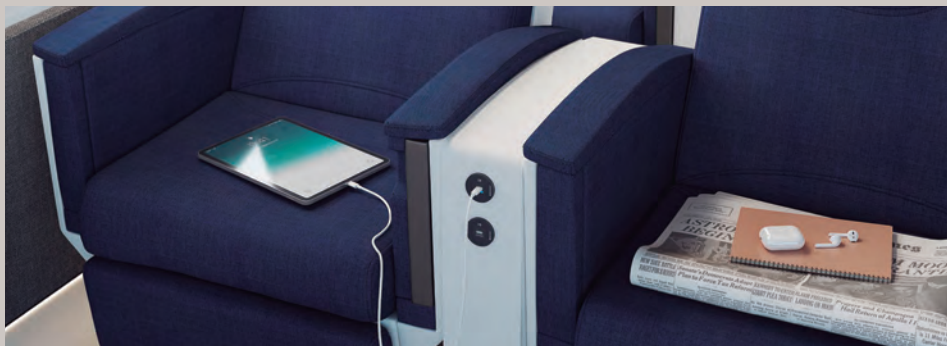
Bit Charger, installiert in einem Zug. Bit Charger installed in the seats of a train.
